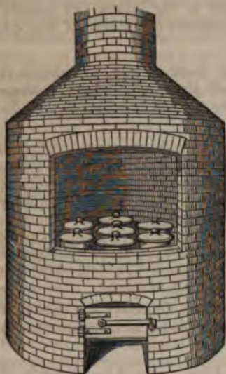
Furnace for the Preparation of Calcined Magnesia.
